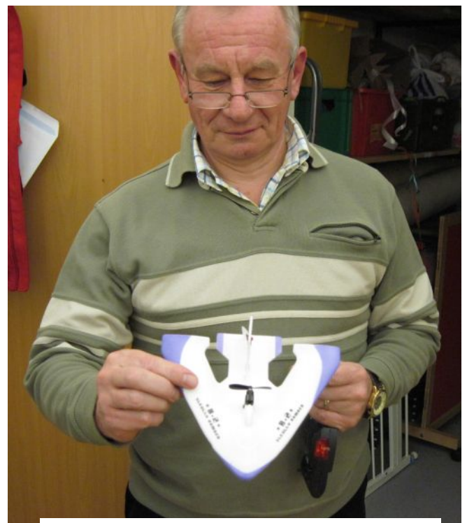
Peter Loxhan examining Noel Starling's unusual Fixed wing model that flew well after some ballast was added to the nose.
